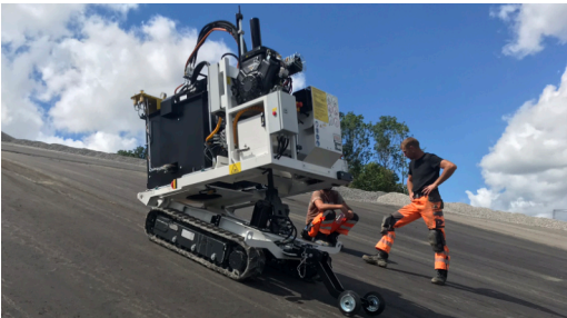
Example projects trailer body according to customer requirements / Hot potting machine for slopes at 33°
